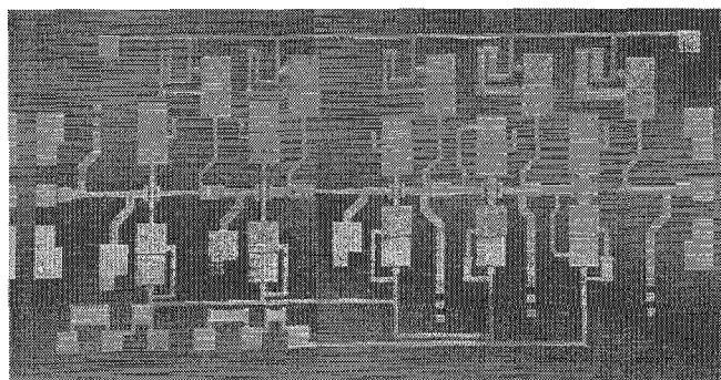
Fig. 2. SEM picture of five-stage Ka-Band low-noise amplifier.
